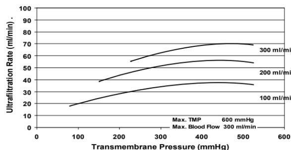
Figure 1: Fresenius HF3000 and HF3000TSB Hemoconcentrator ultrafiltration rates
